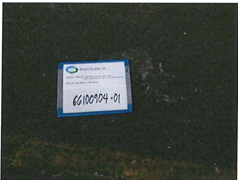
Photo #3: Ground floor. Non-asbestos containing black flooring (asphalt).
