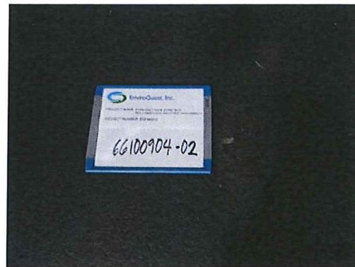
Photo #4: Ground floor. Non-asbestos containing black flooring (asphalt).
